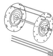
To extract when cooking finished, keep the unlock button (15) to the right and with the handle (12) lift up the accessory and extract it.
